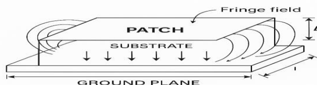
Figure 1: Fringe Field from Patch to Ground Plane
