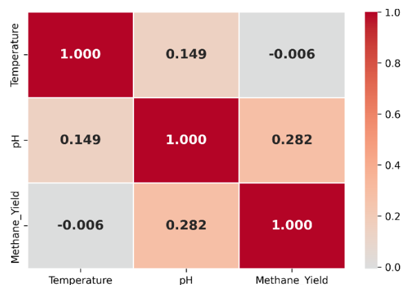
Figure 2: Pearson Correlation Matrix for Temperature, pH, and Methane Yield. Temperature Shows Near-Zero Linear Correlation with Yield ( r = -0.006 ) while pH Shows a Modest Positive Correlation ( r = 0.282 )
