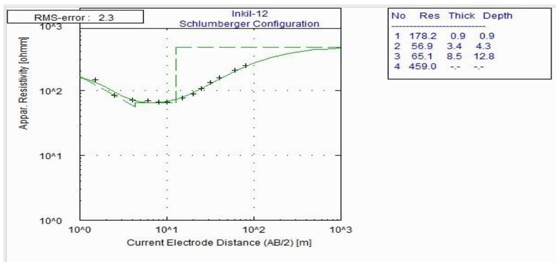
Figure 3: Resistivity model at station 12 (VES 12)
