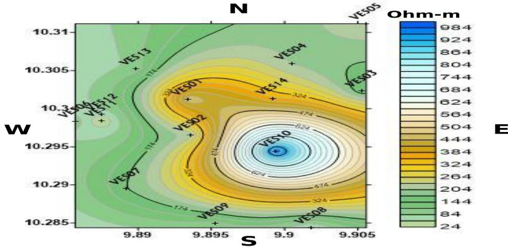
Figure 4: Isoresistivity contour map of the inferred aquiferous zone.
