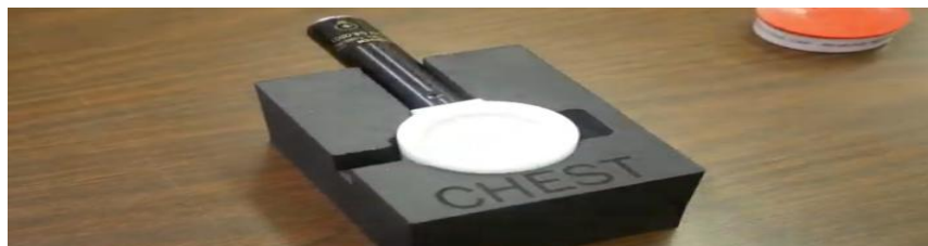
Plate 1: Radcal 10X6-6M Mammography Ionization Chamber in a Chest Block
