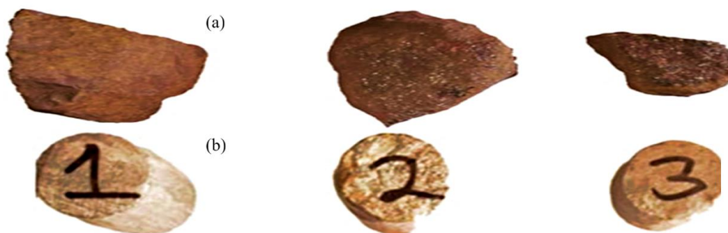
Figure 4: (a) Raw iron ore samples from Itakpe; (b) Cylindrical core prepared for laboratory measurements
