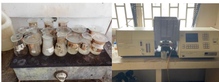
Figure 4: The Prepared Sample and Atomic Absorption Spectrophotometer (AAS)
