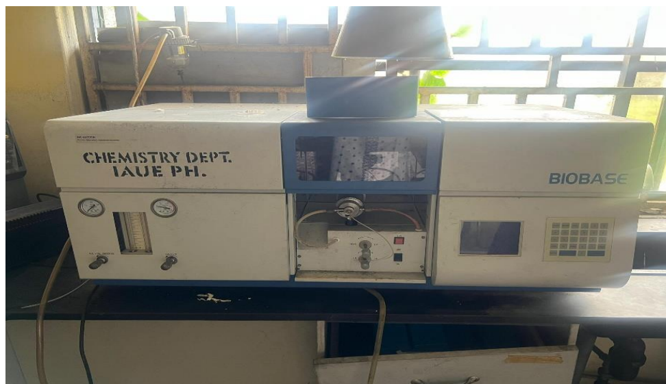
Figure 2: Agilent Technologies Network Atomic absorption spectrometer SN-PGAA 500
