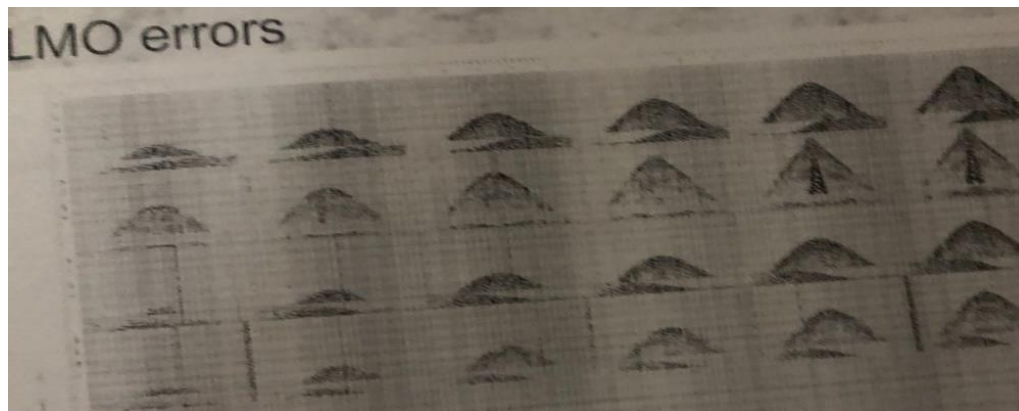
Figure 2a: Showing LMO Errors due to Incorrect Receiver Stations Deployment on the Recorded Seismic Receiver Lines
