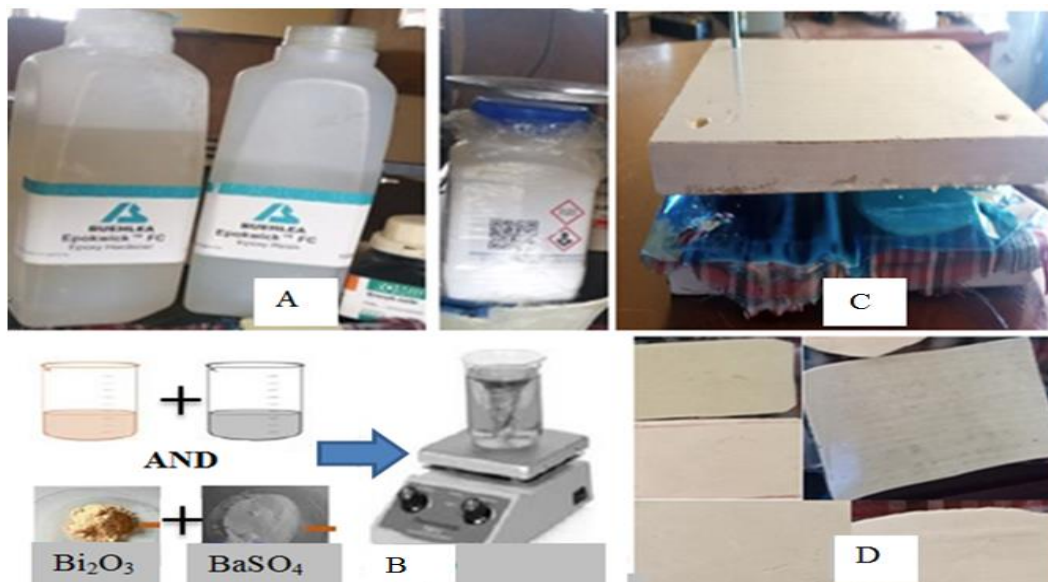
Figure 1: (A) Liquid Epoxy Resin and Micro Powder of Bismuth Oxide and Barium Sulphate. (B) Synthesis of Composite Samples. (C) Cast of Composite Samples. (D) Composite Samples
