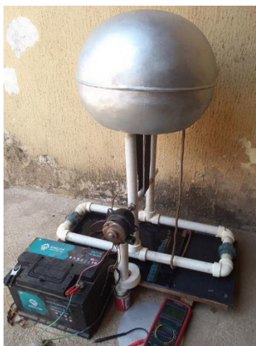
Figure 1: The complete VDG Accelerator built from locally sourced materials
