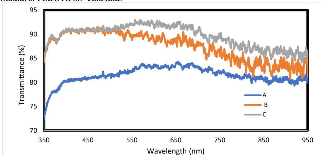
Figure 2: Transmittance spectra of PEDOT:PSS thin films on glass substrate at different temperatures conditions. (A-as-deposited, B- 100 °C , and C- 200 °C)
