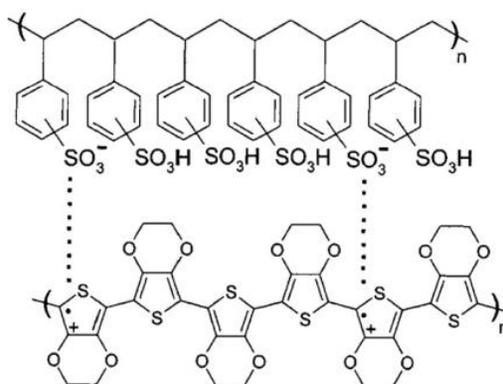
Figure 1: Schematic diagram of PEDOT (up) and PSS (down) Nardes et al., (2008)
