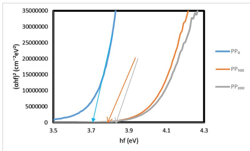
Figure 4: Plots of  $(\alpha hf)^2$  vs photon energy of PEDOT:PSS thin films at different annealing conditions; As-deposited = (PP<sub>0</sub>), 100 °C = (PP<sub>100</sub>), and 200 °C = (PP<sub>200</sub>)
