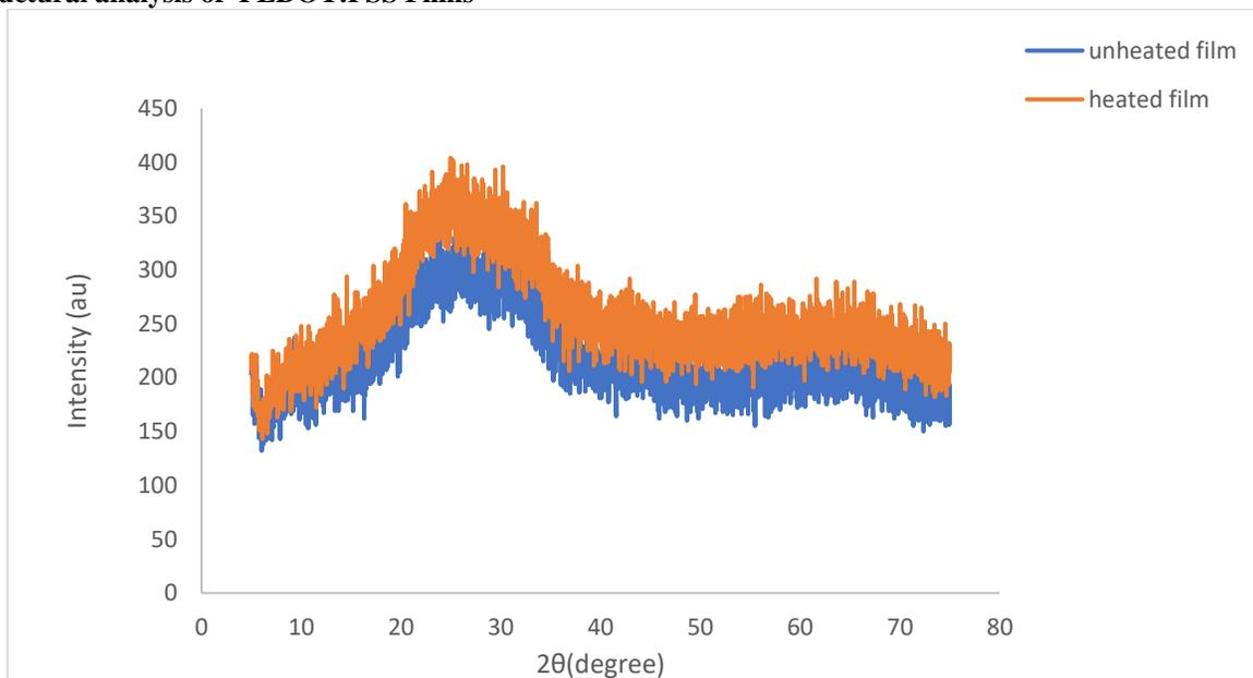
Figure 6: Powder X-ray Diffractometer (PXRD) diffraction of annealed (200 °C) and unannealed PEDOT:PSS films
