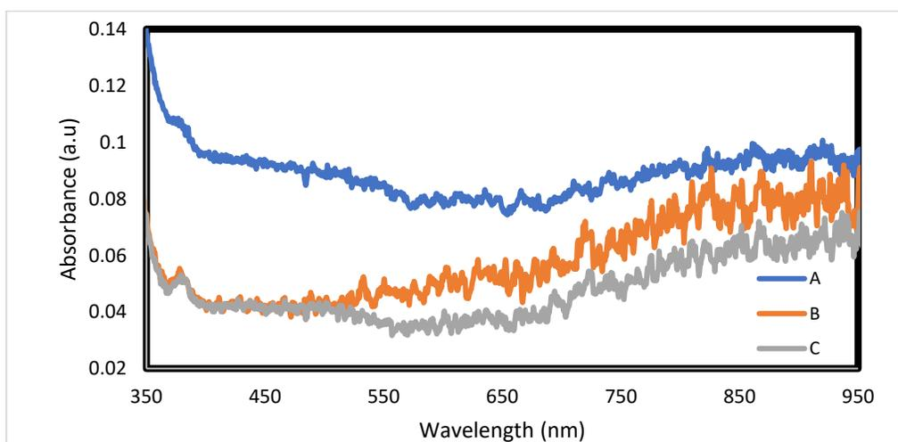
Figure 3: Absorbance spectra of PEDOT:PSS films as a function of annealing temperatures. (A- as-deposited, B- 100 °C, and C- 200 °C)
