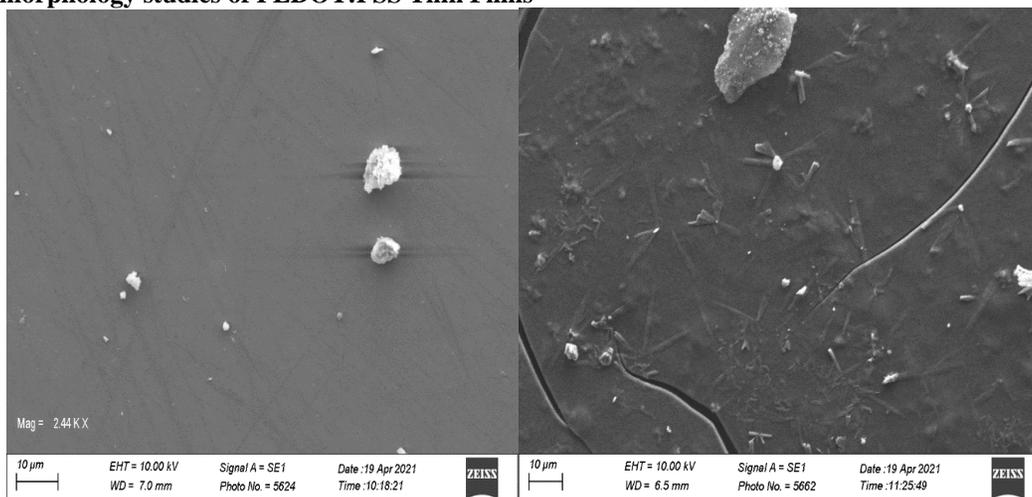
Figure 5: SEM micrographs of (a) Unannealed and (b) annealed PEDOT:PSS films
