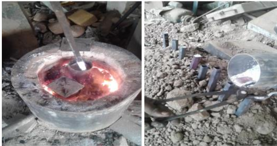
Figure 1: Laboratory stir casting set up for the production of Al-Si alloys
