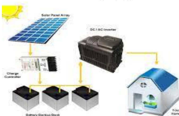
Figure 1: Off-grid Solar PV system
