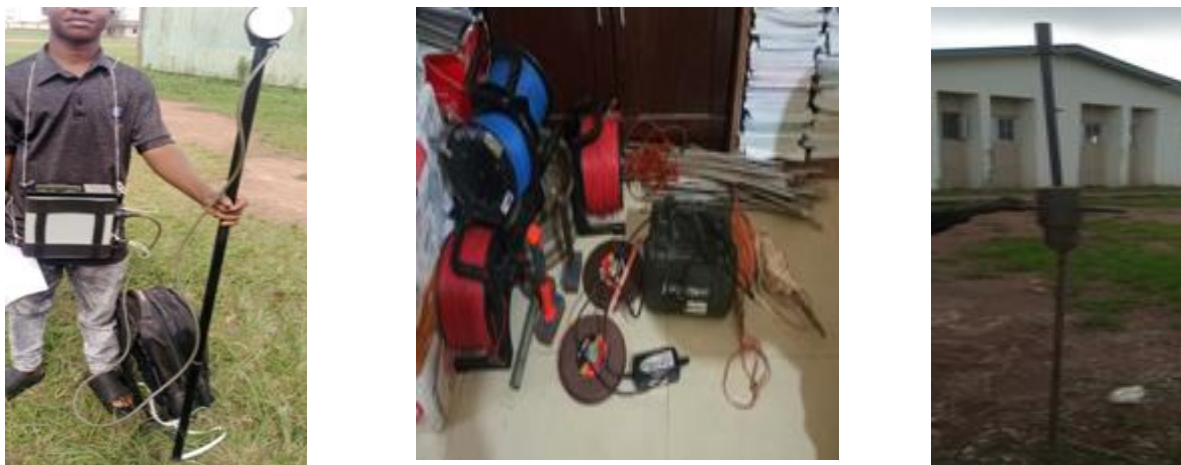
Plate 2: Equipment used for data collection: (a) Proton magnetometer (b) Terrameter and its accessories (c) DCPT apparatus
