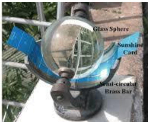
Figure 1: Campbell Stokes sunshine recorder
