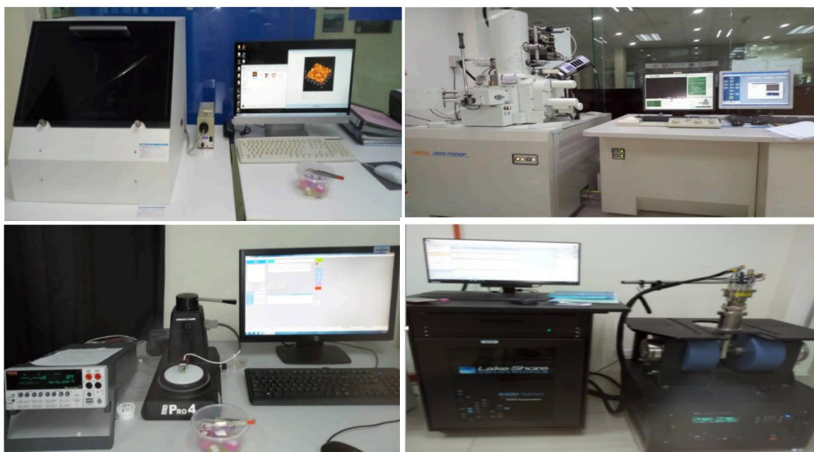
Figure 1: Set-up characterization models for (a) AFM (Topological analysis), (b) FESEM (morphological analysis), (c) Four-point probe (Electrical analysis) and (d) Hall Effect system (Electrical analysis).
