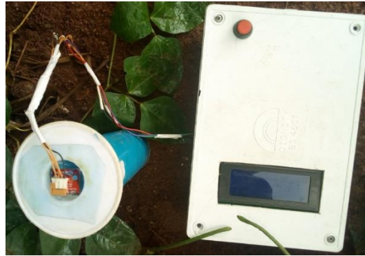
Figure 5: Complete soil infiltration device
