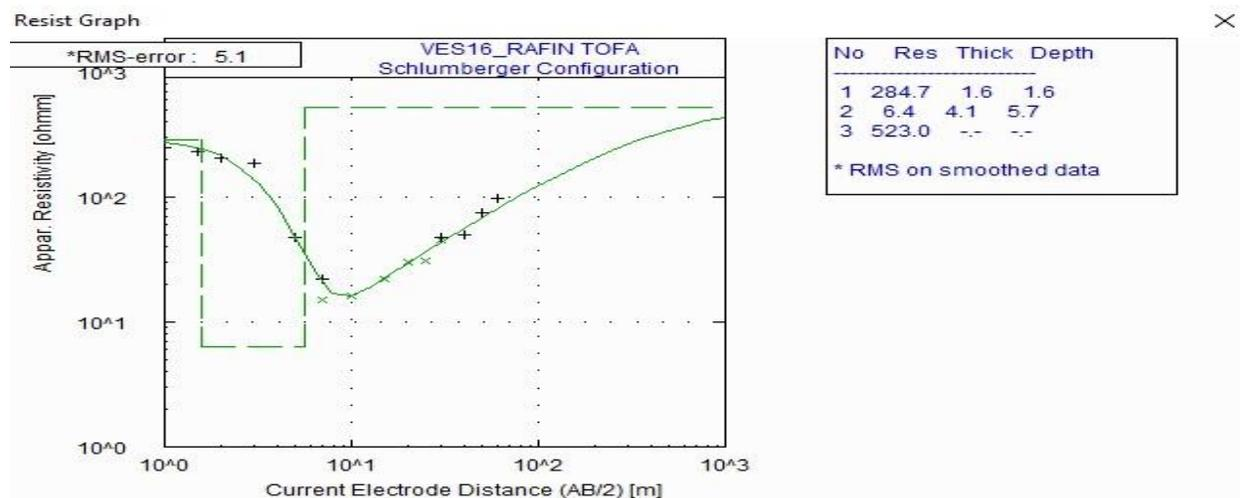
Figure 3: A typical H-Type Curve
