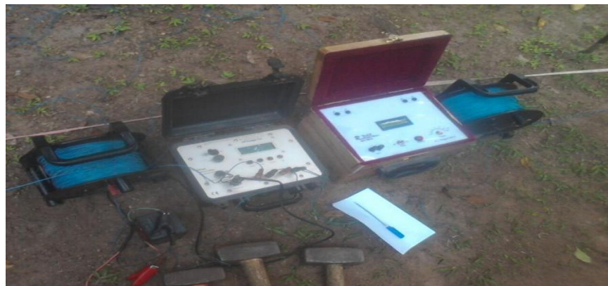
Plate 1: Field Testing using Standard and Fabricated Resistivity Meter
